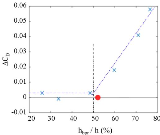
Figure 11.  $\Delta C_D$  vs  $h_{bpr}/h$  for Configuration IV relative to I. Baseline in red.
