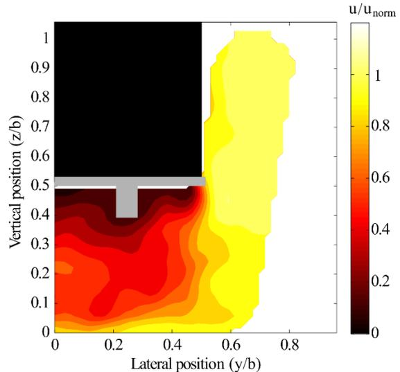
Figure 12. Normalised streamwise velocity contours on plane  $x/b=6.35$  for configuration with no bumper.
