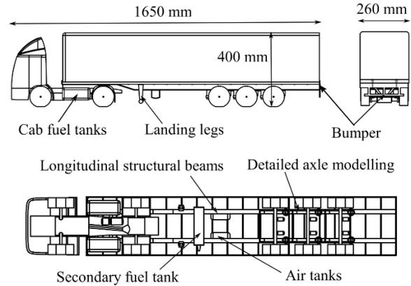
Figure 4. 1/10<sup>th</sup> scale model (in mm).
