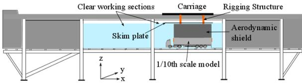
Figure 2. Water tow-tank and model installation. The coordinate system is labelled.
