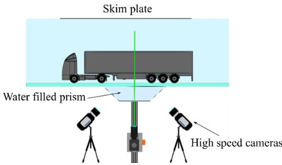
Figure 9. Stereoscopic PIV setup.
