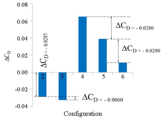
Figure 14.  $\Delta C_D$  for configurations II-VI relative to the baseline for  $h_{bpr}/h = h_{ss}/h = 76.5\%$ .
