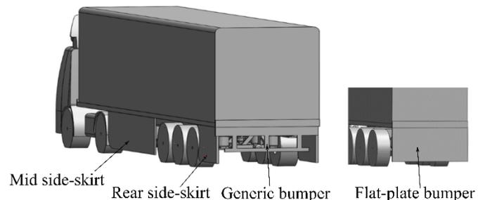
Figure 1. CAD schematic of lorry model with mid and rear side-skirts and generic and flat-plate bumpers.
