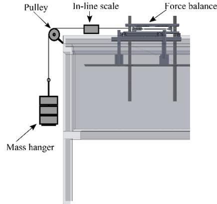
Figure 8. Load cell calibration setup.
