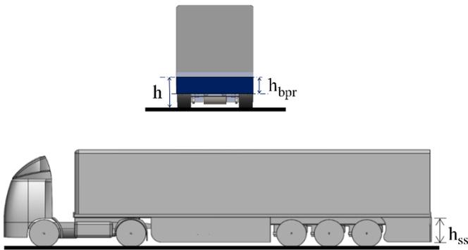
Figure 6. Flat-plate bumper and mid and rear side-skirts tested for range of normalized heights.
