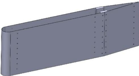
Figure 3. CAD schematic of aerodynamic fairing.
