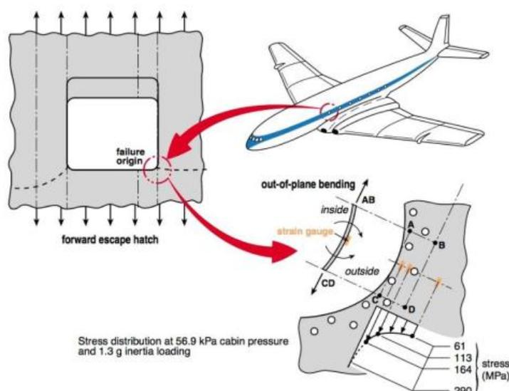
Aircraft fuselages, like any cylindrical shape, develop internal membrane stresses to resist the internal pressure loads. These forces induce secondary out-of-plane bending moments trying to “straighten-out” the curve.
