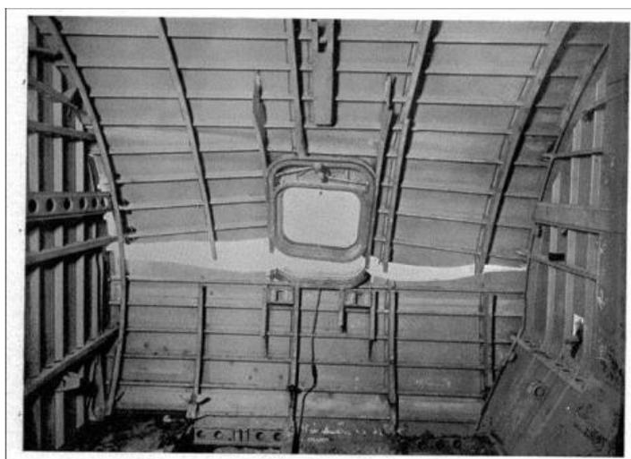
Fatigue cracking was found that originated from the rear lower corner of the forward escape hatch, and also from the right-hand aft corner of windows. In tests on another Comet aircraft, investigators had found that up to 70% of the aircraft's ultimate stress under pressure was concentrated on the corners of the aircraft's square windows. (Withey, 1997)
