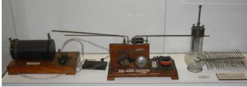
Figure 1: Hülsmeyer's Telemobiloscope [3]
