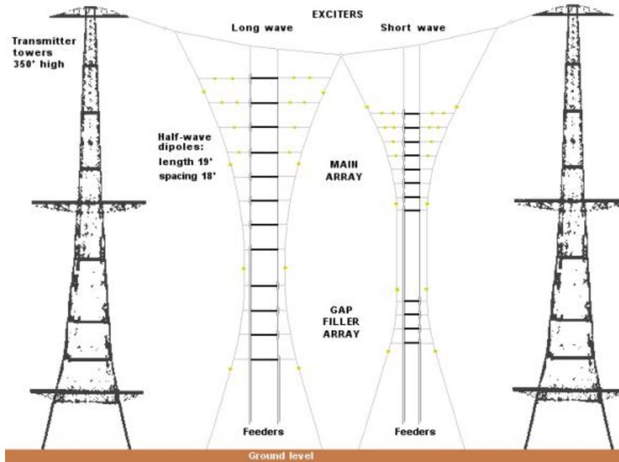
(a) Diagram of Chain Home transmit antennas [15]
