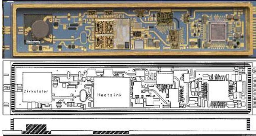
Figure 11: A single T/R (transmit/receive) module from the CAPTOR-E programme with diagram annotated in German. The antenna connection is on the left; the circulator (Zirkulator) isolates the transmitter from the receiver. The two darker coloured chips in the centre of the photograph are the transmit power amplifier transistors. The whole unit is only 64.5mm long. [50]
