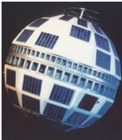
(a) Telstar. Note the helical antenna at the top of the spacecraft.
