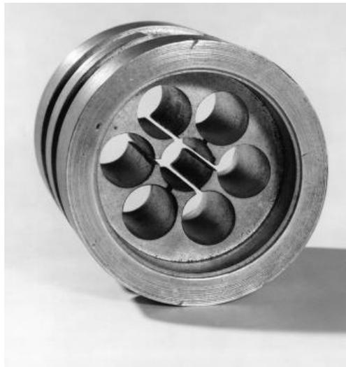
Figure 7: Randall & Boot’s original 1940 magnetron core, showing cavities. [19]
