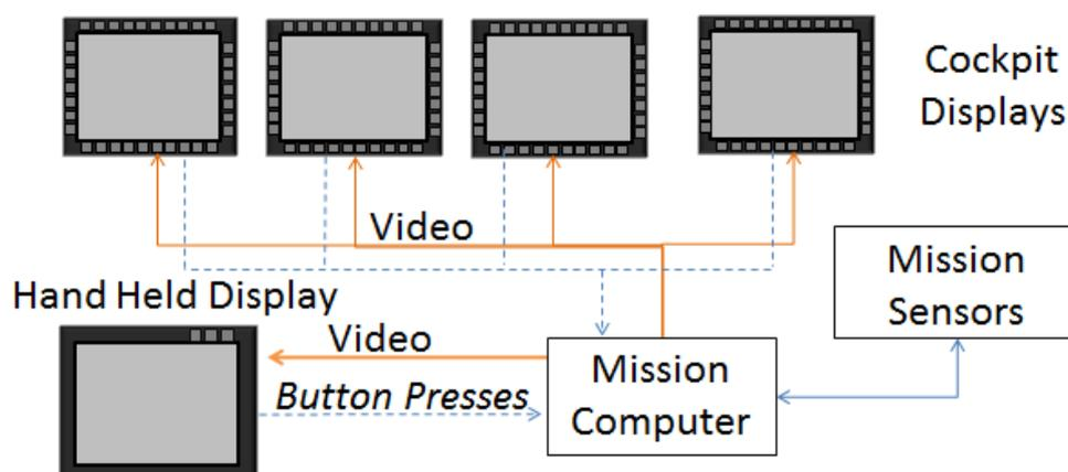
Figure 3: Proposed mission display integration solution
