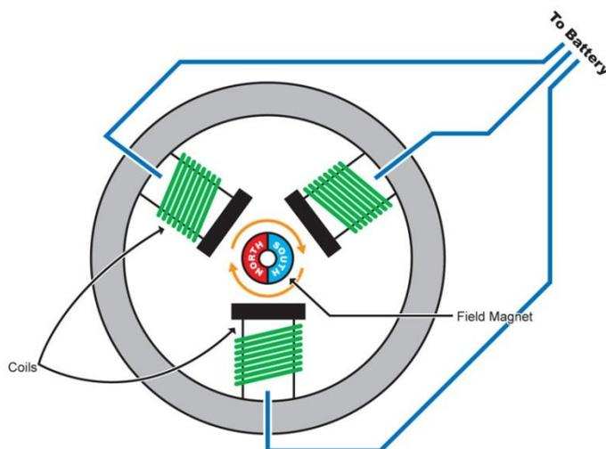
Figure 6: Simplified Diagram of Brushless Motor [7]
