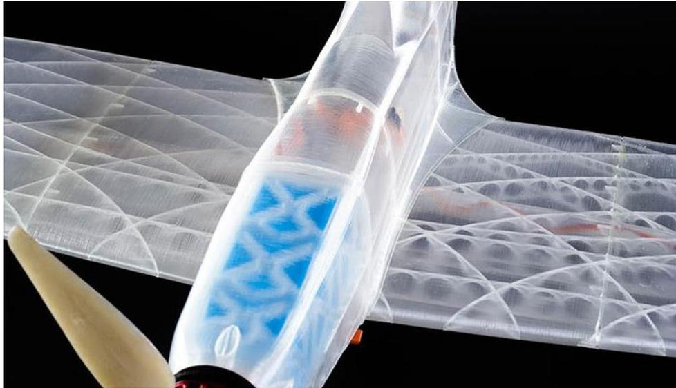
Figure 2: 3D Printed Small UAV with Internal Wing Structures [3]
