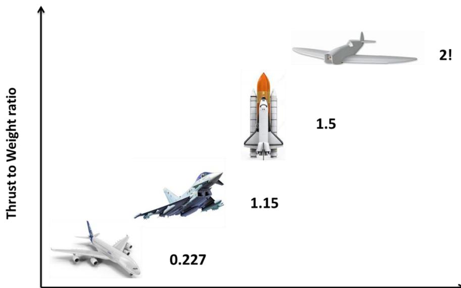
Figure 3: Thrust to Weight Comparison of Different Aircraft Types [4]
