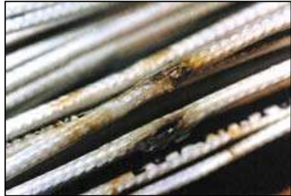
*Figure 8: Wire chaffing due to vibrations [19]*
