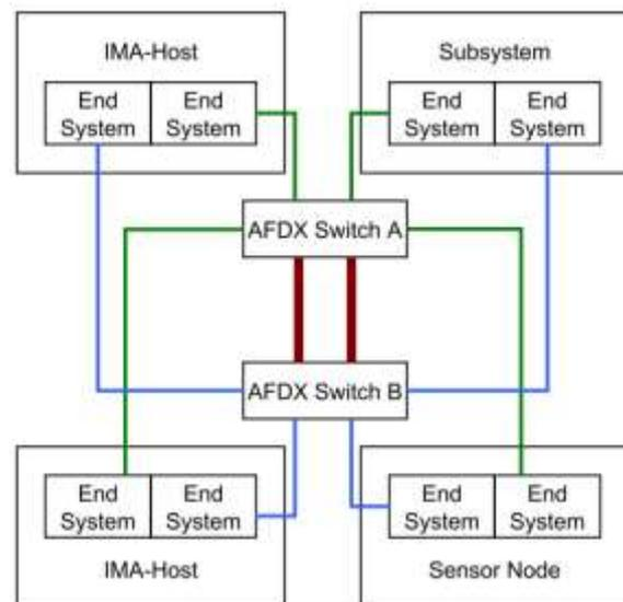
Figure 5: AFDX Topology example [13]
