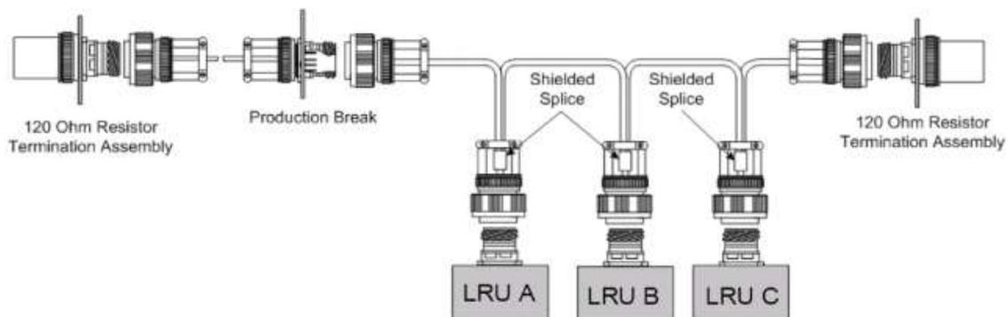
Figure 2: Typical design of CAN bus installation in an aircraft [2]
