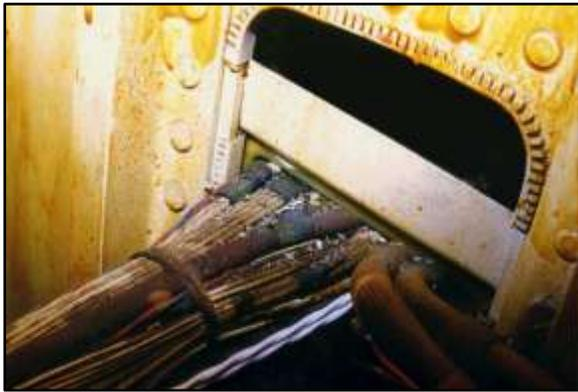
*Figure 9: Wire aging in aircrafts [18]*
