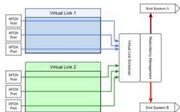
Figure 6: Virtual Link layout in the AFDX network [13]
