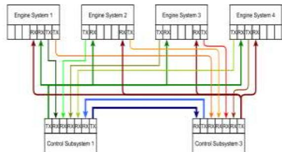
Figure 3: Complexity of the ARINC 429 system containing only two controlling subsystems and four data-consuming components [3]
